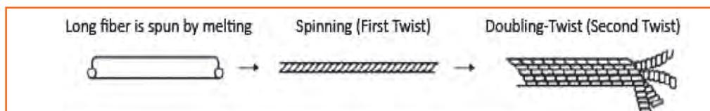
Fig.2.1.87 (a): Thread Structure
