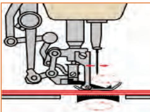
Fig.2.1.18: Unison Feed Mechanism
