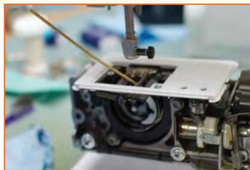
**Step 2:** Check feed dogs: Remove the feed dog, clean the feed dogs. Try to pass a rag under them and with an old needle or narrow tool, remove the lint inside the feed channels. Put back the needle plate. If your machine is equipped with a FEED DROP, be sure the feeds are set at UP position. By turning the hand wheel (towards you), check to see if the feeds make their movement.
