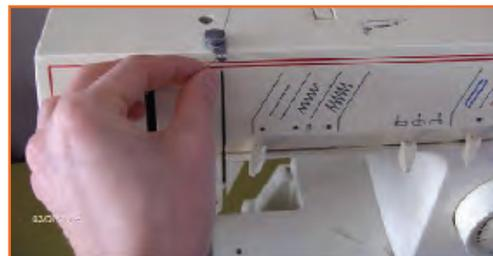
**Step 4:** From the tension bring the thread up and from right to left put it through the hole here.
