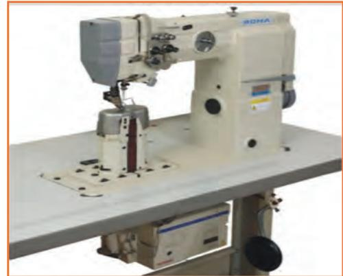
Fig.2.1.4: Post-bed Sewing Machine
