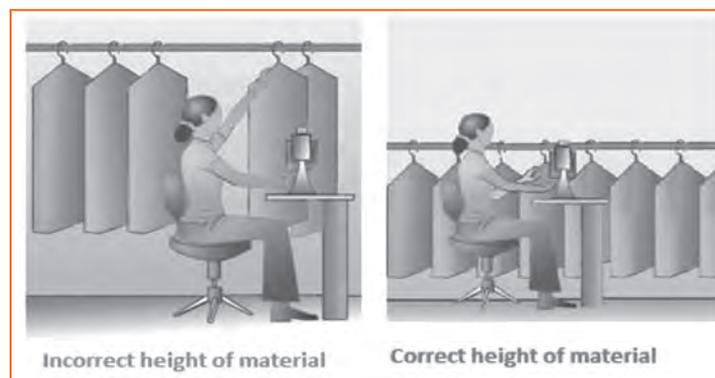
Fig.5.1.4: Situating the material
