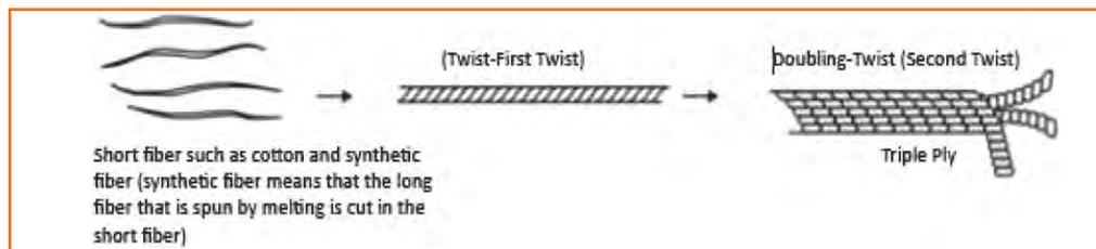
Fig.2.1.87 (b): Thread Structure
