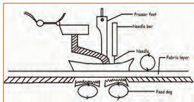
Fig.2.1.16 (b): Differential Bottom Feed Mechanism
