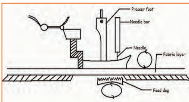
Fig.2.1.16 (a): Differential Bottom Feed Mechanism
