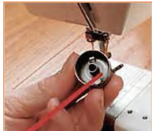
Fig.4.1.2: Cleaning the bobbin and case
