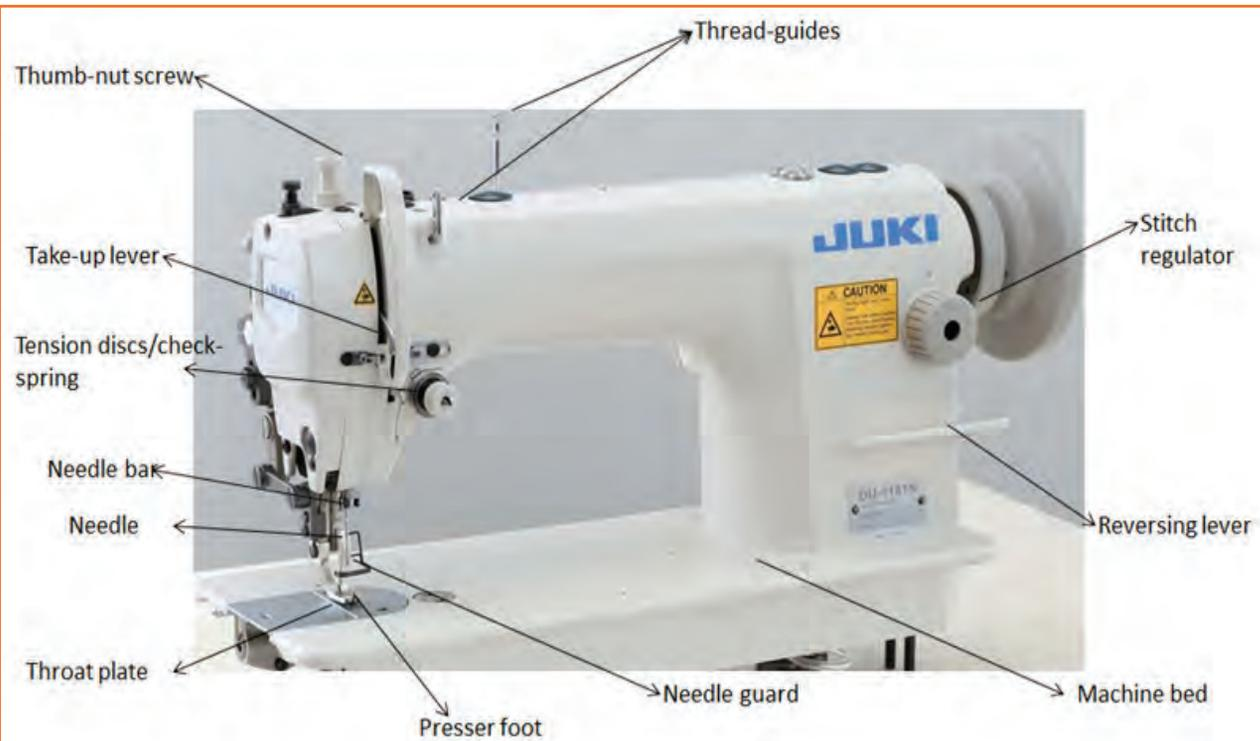
Fig.2.1.20: Parts of a Sewing Machine
