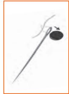
Fig.2.1.72: Needle threader
