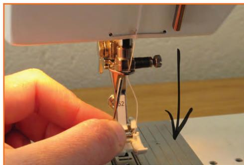
**Step 2:** Remove the needle by pulling down and away from the needle clamp.
