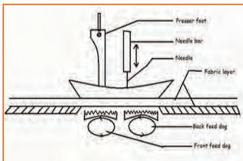
Fig.2.1.15: Differential Bottom Feed Mechanism
