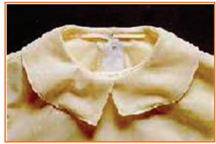
Fig.3.1.22(c): Interlining shrinking
