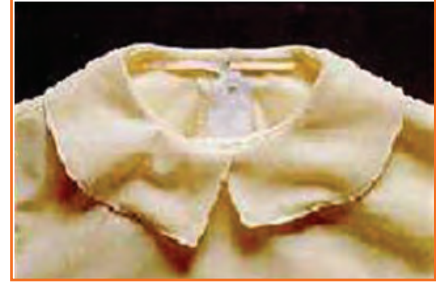
Fig 3.2.17(c): Interlining shrinking
