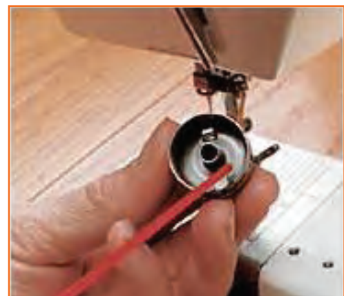
Fig 4.1.2: Cleaning the bobbin and case
